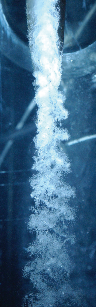
ABOVE Axisymmetric, turbulent bubbly wake resulting from the collapse of a ventilated supercavity.
