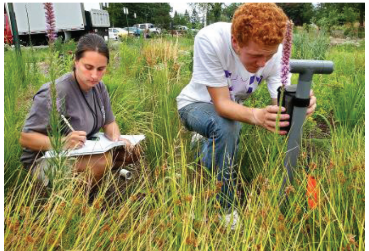
Graduate student Brooke Asleson and undergraduate research assistant Tom Natwick use a soil moisture probe to determine how saturated the soil is in the UMD rain garden. Photo courtesy of Bob King/Duluth News Tribune.
