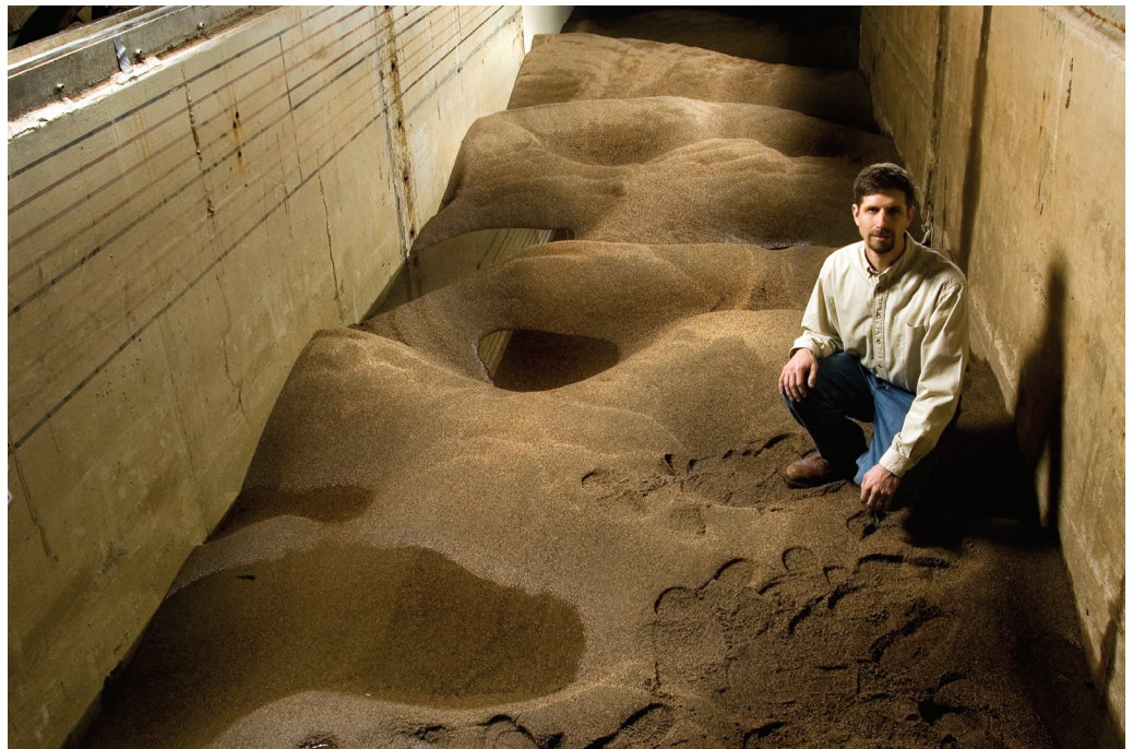
StreamLab Project Manager Jeff Marr. The Main Channel is capable of recirculating sand and gravel, and continuous monitoring of sediment flux. The facility will be used for community-wide, integrative research on physical, chemical and ecological processes in stream.
