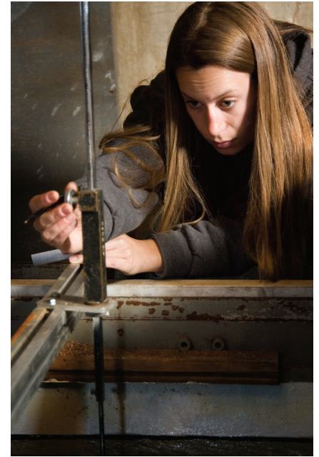
Research scientist Sara Johnson takes water surface measurement with a point gage during a StreamLab experiment.
