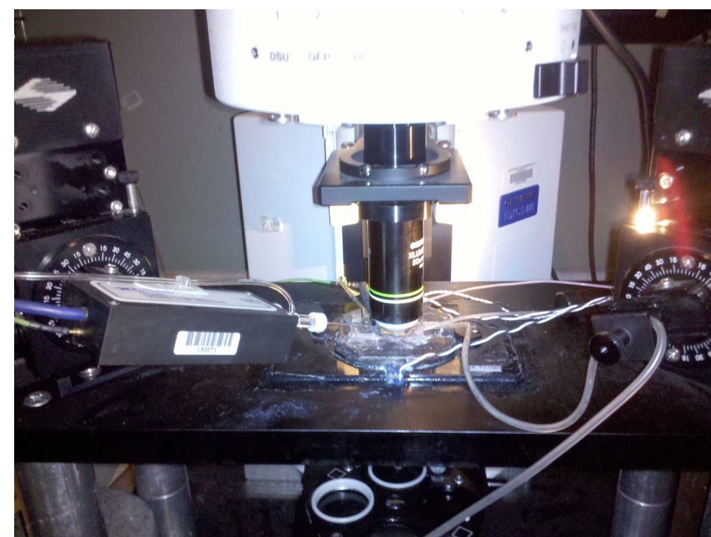
Figure 2. Experimental setup. The slice is placed in the center underneath the microscope, with the electrode mounted in the manipulator on the left. The image is projected onto a television screen (not shown) for better view.
