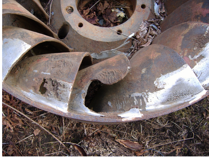
FIGURE 1.1: Cavitation damage to a Francis turbine, with large sections of the blades completely worn away [10].
