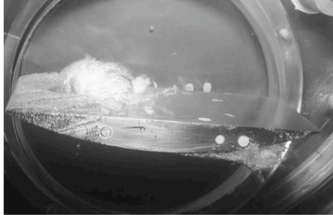
FIGURE 1.2: Transition from sheet-to-cloud cavitation (Callenaere et al. [12]). Flow is from left to right.
