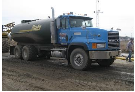
S5 (Homemade 4,400 gal – flotation tires)
