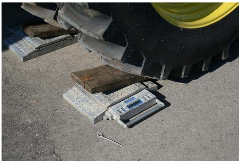
Figure 2.15. Weighing vehicles using portable scales
