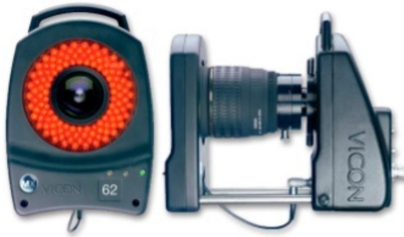
Figure 2.3: The 4 mega pixel MX-40 Vicon camera operates at frequencies up to 166Hz (frames per second). Near infrared LED light (red ring in image) was used to enhance the tracking performance of the six cameras installed in the lab (taken from Mettler (2010)).
