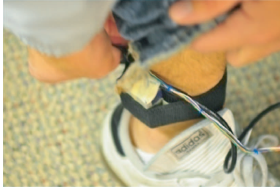
Figure 2.7: Photo of the Microbotics, Inc. MIDG II INS/GPS sensor [21] secured to an elastic band and worn above the ankle. Data from the MEMS accelerometers inside the MIDG are used with the kinetic model to estimate step size in-situ.
