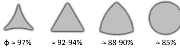
Figure 2.2. Ligament cross-section as a function of porosity [25].
