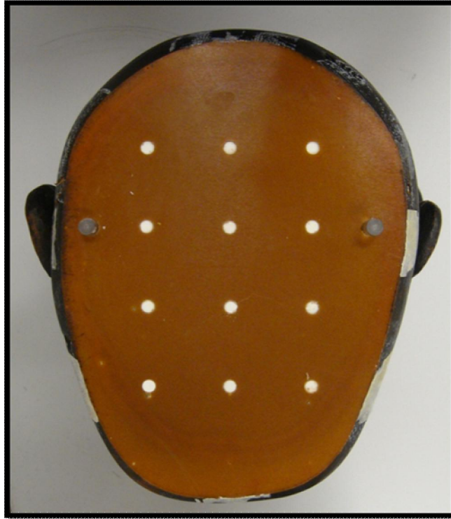
Figures 2 and 3: Example of phantom axial slices with grid holes for TLD placement
