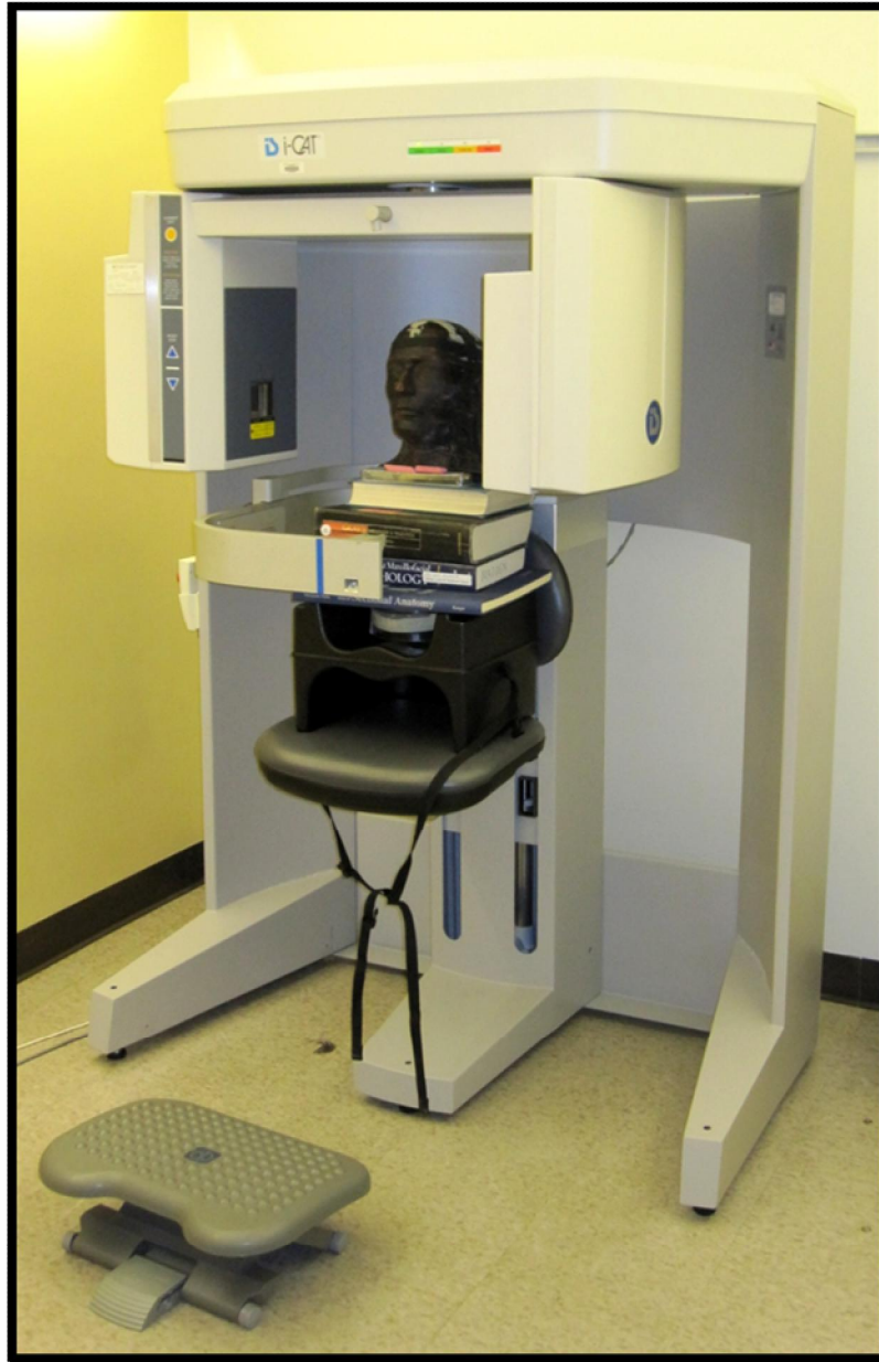
Figure 5: Set up of phantom in proper scanning position within the NextGeneration iCAT CBCT machine
