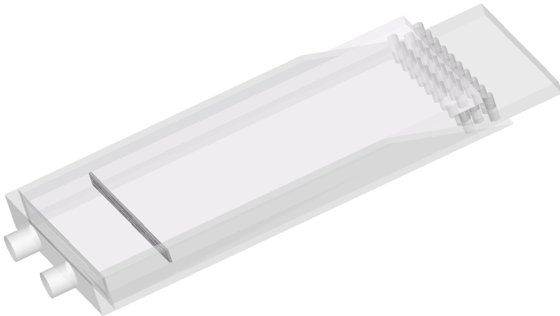
Figure 3.11. Coolant plenum with installed turbulators.
