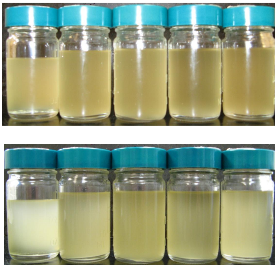
Figure 3.9: B-side Compatibility tests of four different surfactants, from left to right: control A, SBOP A_3805, SBOP A_7105, SBOP A_8404, SBOP A_9204 (top) mixture of polyol, water, catalyst, surfactant and n-pentane; (bottom) mixture of (top) with addition of glycerol for SBOP A mixtures.
