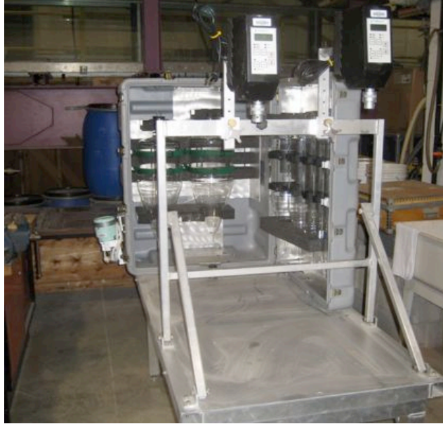
Figure 3.2. Portable elutriation device developed by Environment Canada.
