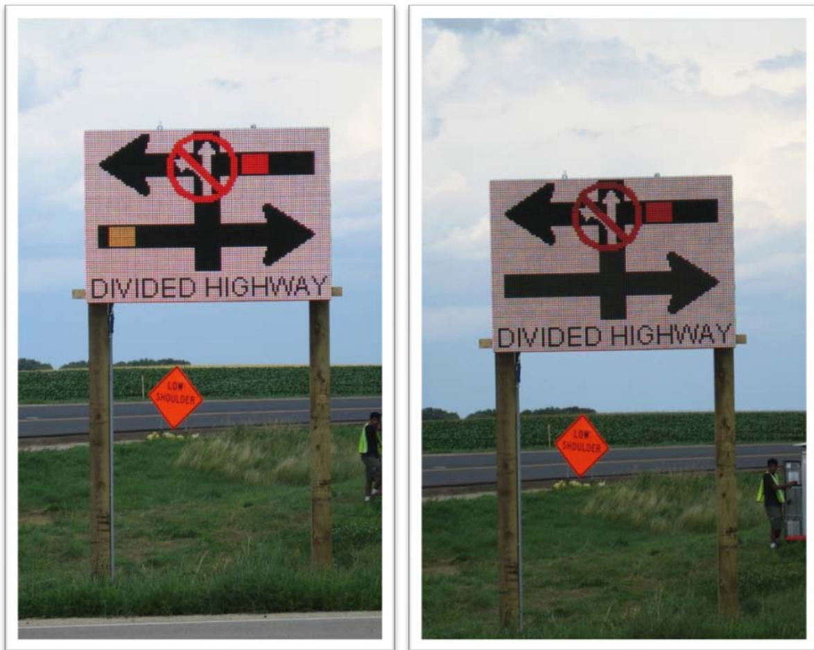
Figure 2. Prototype DIIs as tested at the Minnesota Research intersection at US 52 and CSAH 9 in Goodhue County, MN. The DIIs are 80x112 pixel, 20 mm pitch LED displays measuring 63in by 88in. In the left photo, traffic approaching from the left is more than 7.5 seconds from the crossroads; traffic from the right is less than 7.5 seconds from the crossroads. In the right photo, the nearest vehicle on the left is more than 11.5 seconds from the crossroads; the vehicle approaching from the right is less than 7.5 seconds from the crossroads.
