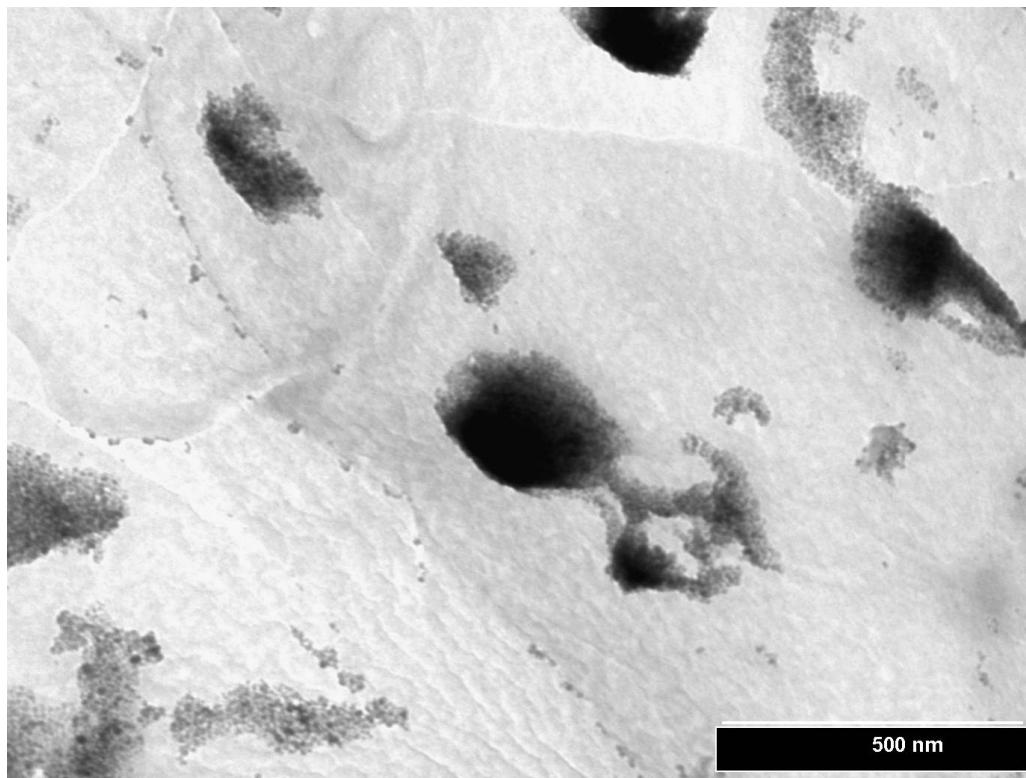
Figure 5-9: TEM of UMB- SPNs-CA nanoparticles on 400 mesh grid at magnification x75,000.
