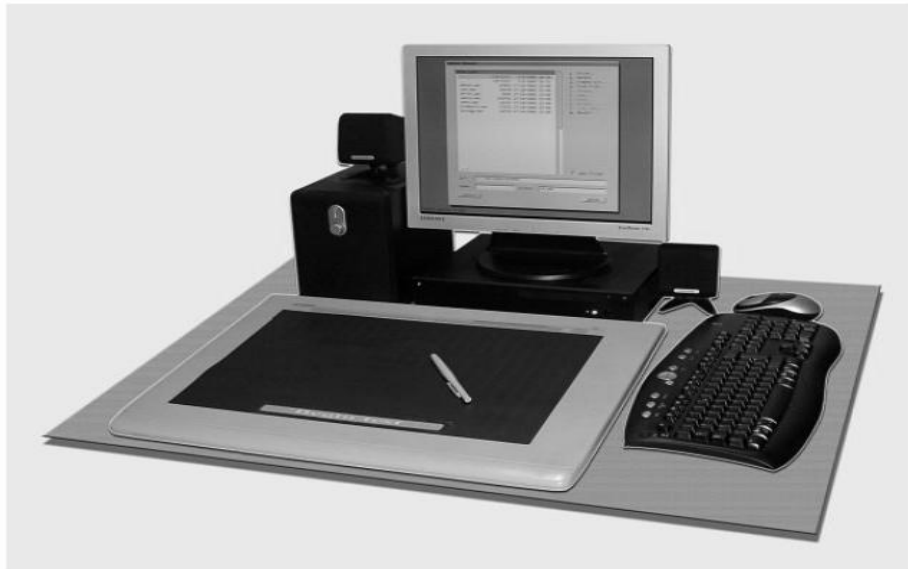
Figure 4. OASIS equipment with Wacom Ultrapad digitizing tablet and electronic pen. Copyright 2007 by Kikosoftware, Inc. Reprinted with permission.
