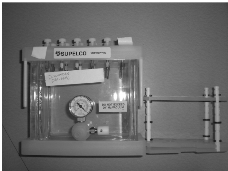
Figure E.3. Vacuum Manifold with Rack
