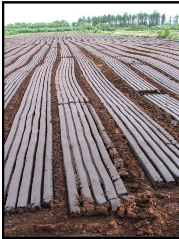
Figure 7:5. Extruded peat from industrial harvesters, Fletcherstown bog, Co. Meath.
