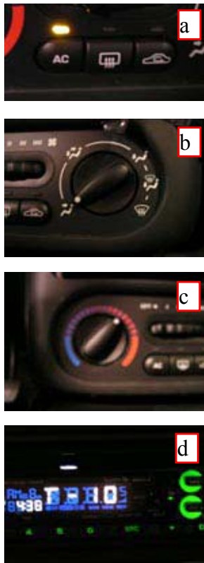
Figure 2-2 – In-Vehicle secondary-task categories, a. Buttons with indicator light, b. Air flow, c. Temperature setting, and, d. CD track
