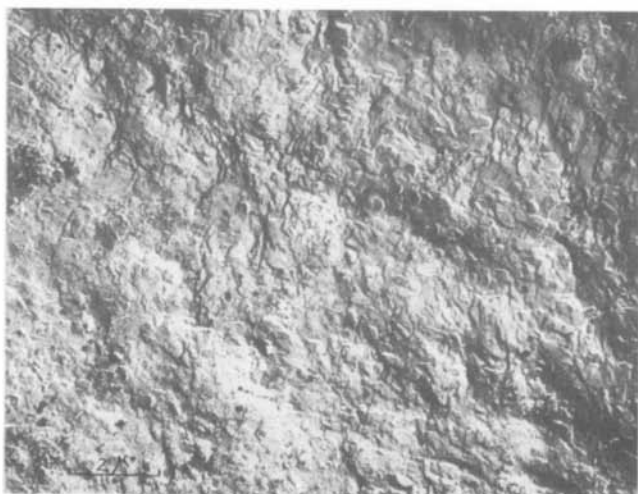
Figure 9--Electron micrograph of a replica of a slickenside surface in Decorah shale. The clay minerals show a high degree of preferred orientation on slickenside surfaces.
