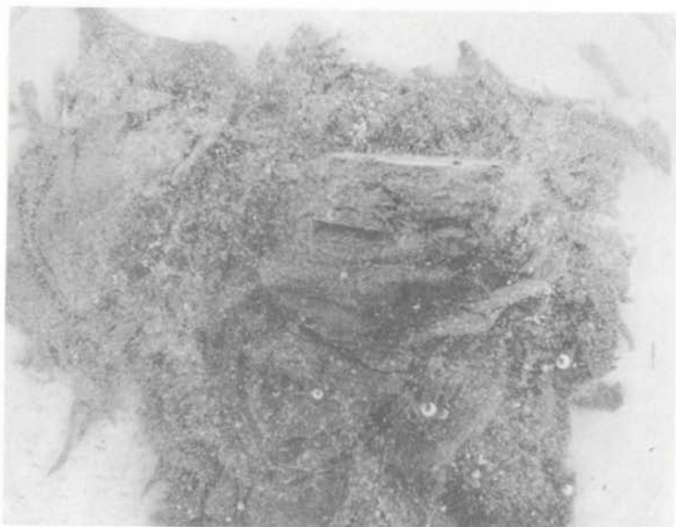
Figure 11-C. Decorah shale sample after 45 seconds elapsed time under water. Note that original bedding surface is still preserved because of its impermeable nature.
