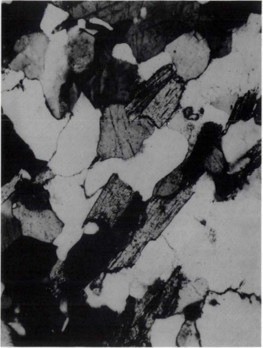
Figure 1 – Crystalloblastic texture of granitic gneiss. The rock is composed of quartz, plagioclase, microcline, and biotite. Sample M8115, (x 65, crossed nicols).
