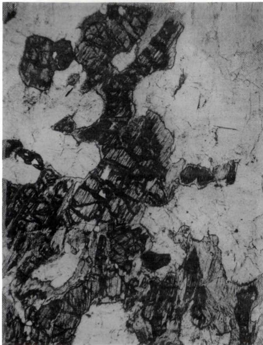
Figure 5 – Hornblende-pyroxene gneiss. Orthopyroxene is partly replaced by serpentine along fractures, and is mantled by cummingtonite. Note that serpentine does not extend into cummingtonite. Sample M8274 (Plane light; x 25).
