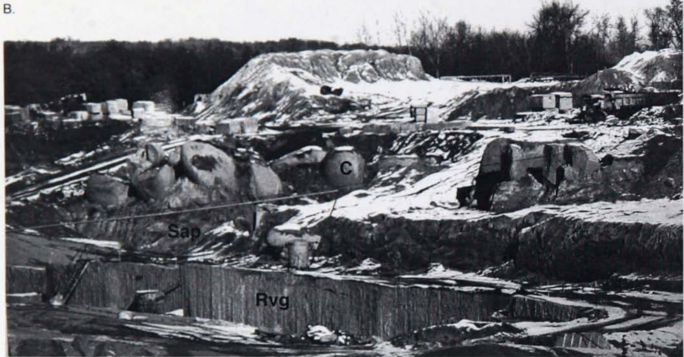
B. Rockville Beige quarry (Stop 4-2B) showing corestones (C) in saprolite (Sap) on top of unweathered Rockville Granite (Rvg).
