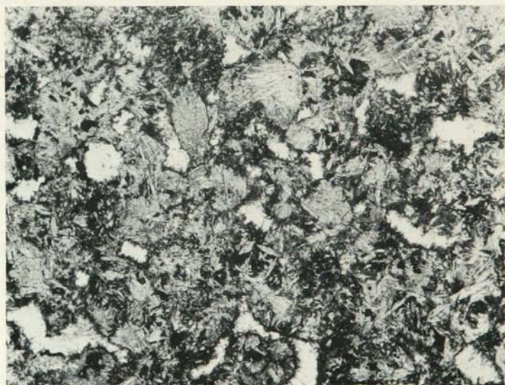
FIGURE 17.—Development of grunerite in stilpnomelane granule taconite in moderately metamorphosed Biwabik Iron-formation (Zone 3). Ordinary light, 21x. The original granules are largely replaced and somewhat obscured by grunerite (light gray), which occurs as small fibrous sheaves and as lath-shaped crystals that cut through the granules. A small amount of pleochroic brown stilpnomelane (dark gray) remains between the crystals. Magnetite (black) replaces the rims of the two granules at upper left, and apparently coexists with the quartz matrix (white) without reaction. FIGURE 18.—Destruction of granule texture of cherty taconite through replacement by metamorphic grunerite in moderately metamorphosed Biwabik Iron-formation (Zone 3). Plane-polarized light, 21x. Original silicate-bearing granules in a quartz matrix (white) are replaced by fibrous grunerite (light gray), which truncates the original granules. A minor amount of magnetite (black) is present.
