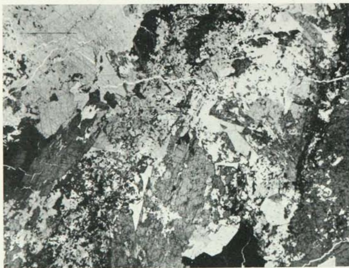
FIGURE 22.—Coarse-grained hedenbergite-calcite veinlet in cherty taconite in highly metamorphosed Biwabik Iron-formation (Zone 4). Plane-polarized light, 4.5x. The veinlet consists of large, partly replaced anhedral hedenbergite (gray), together with coarse calcite (light gray, upper left), quartz (white), and pyrrhotite (black). Minor amounts of magnetite and fibrous green amphibole are present. The diagonal black band at the right consists of fine-grained magnetite and is continuous with similar layers in the enclosing cherty taconite, indicating that the coarse-grained veinlet has developed by replacement of the taconite.
