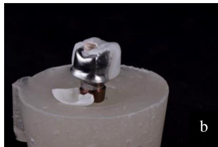
Figure 10. Example of fracture failure of (a) CR, (b) MA, and (c) HA specimens
