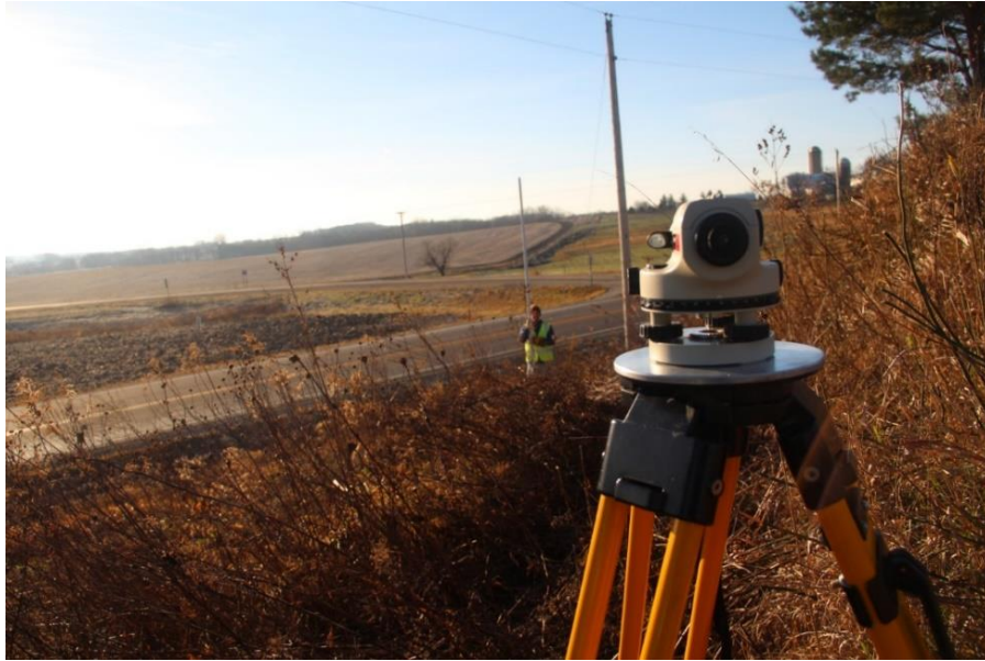
Figure 14: Field survey equipment used to determine slope geometry
