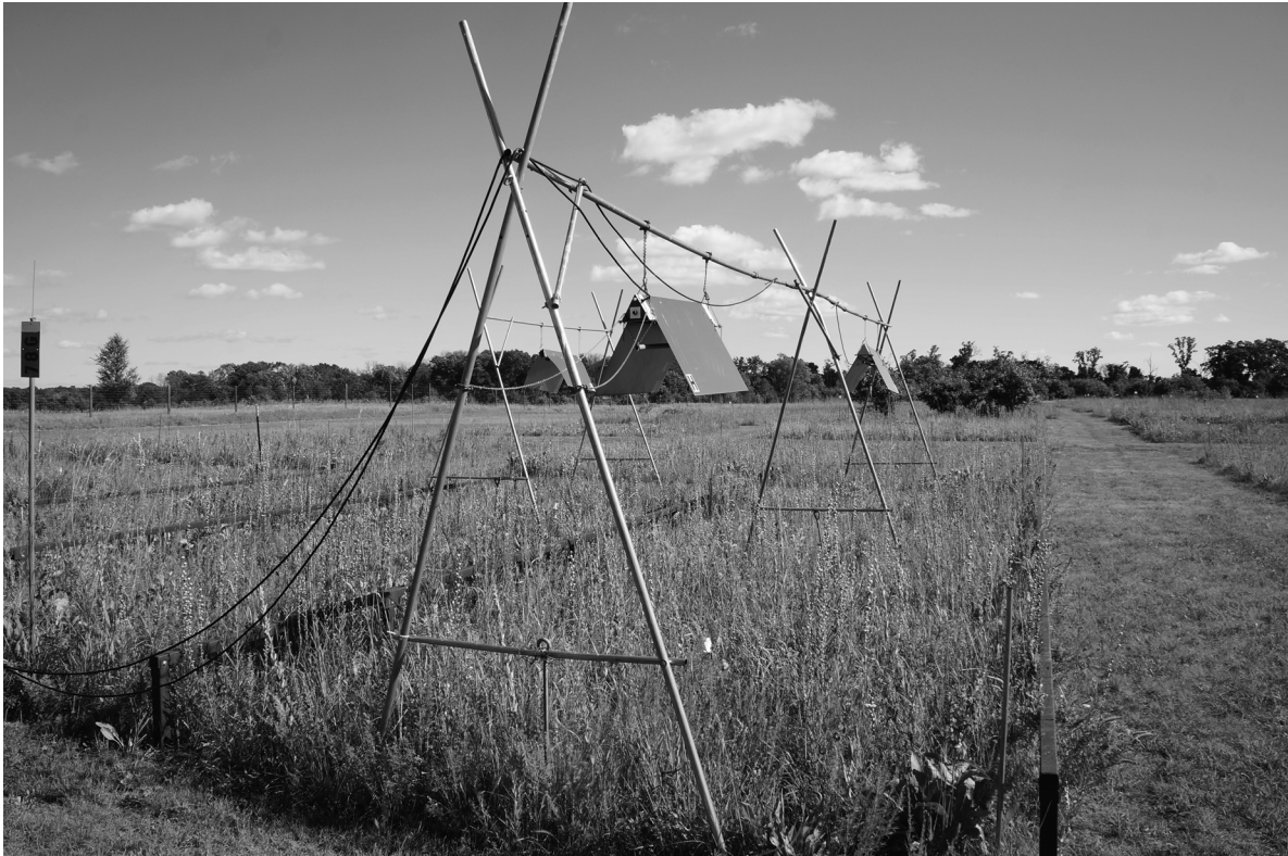
PLATE 1. High plant diversity plot within the BAC experiment established at the Cedar Creek Ecosystem Science Reserve, Minnesota, USA, for studying warming effects on a grassland ecosystem. Metal flanges and frames with infrared lamps were hung over all subplots to increase the temperature by either 1.5°C or 3°C, and hung as well as above control subplots to account for shading effects. Photo credit: K. Steinauer.
