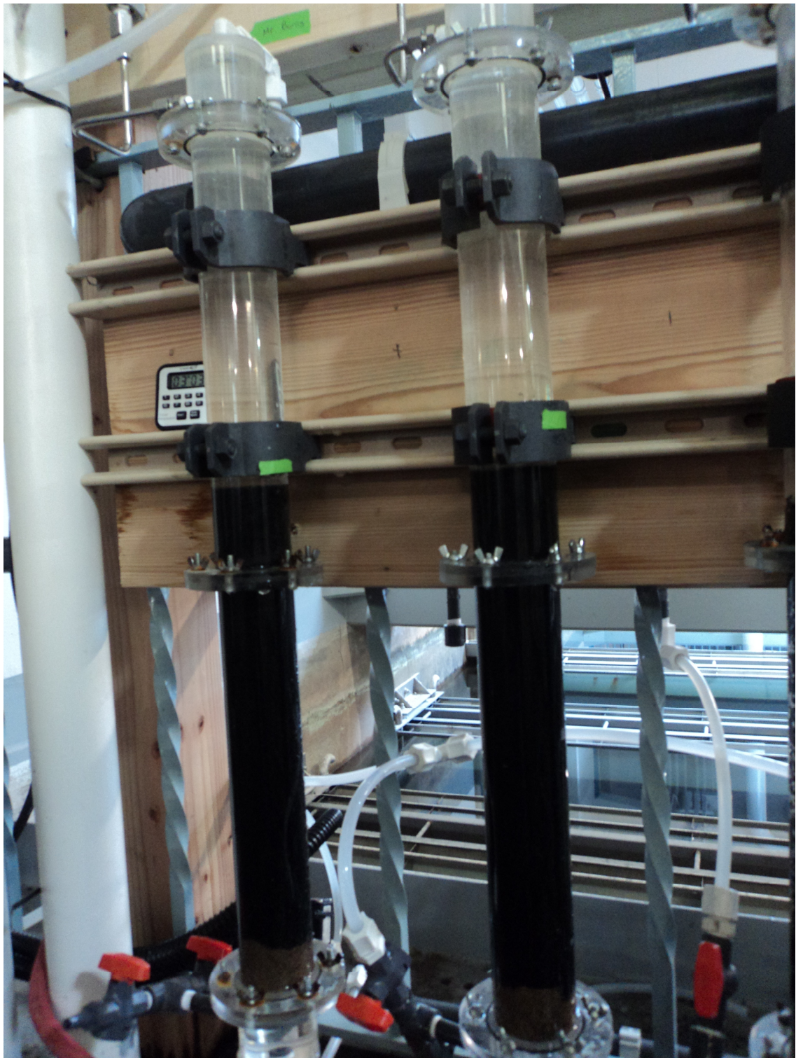
Figure 6-5: Close-up of two columns, notice bottom layer of sand supporting GAC media.
