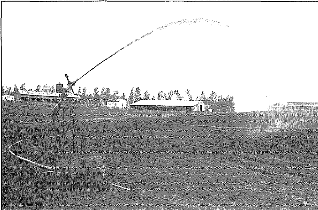
Figure 8. Traveling-gun irrigation unit applying liquid sewage sludge to grass treatment areas.
