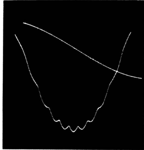
Figure 2.3.2: Experimental data of Little and Parks. Top trace shows the magnetic field swept from high to low. The bottom trace shows the T_c variation during the sweep.[61]
