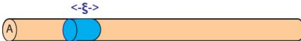
Figure 2.2.1: Blue region of nanowire is normal during a phase slip event.
