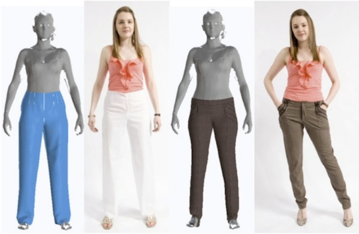
Virtual block fitting/ Physical block fitting/Virtual design fitting/Physical design fitting Figure 2: Trouser project process
