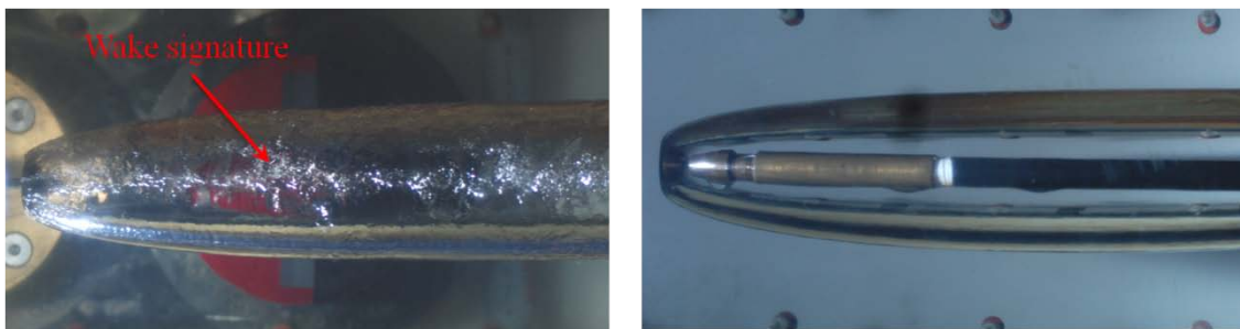
Figure 2.3.8: Comparison of supercavities created by the two models. Left: backward facing model. Right: forward facing model.
